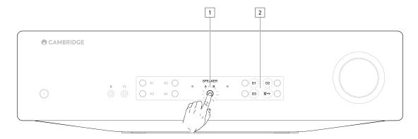
**Note:** Press the Speaker A/B button once to leave the Setup menu and place the CXA back into Standby mode.
