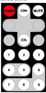
**POWER** turns the unit on or back into standby
