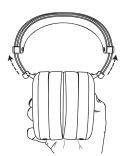
Move the sliders up until the leather is against the titanium headband.
