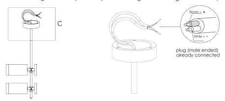
After inserting the cables into the space inside the plate, screw the model to ceiling by using the three screws provided, checking that it is securely and stably fastened.
