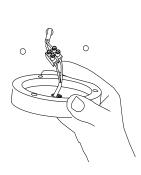
Once screwed in (and by getting help from another person), mark the 3 ceiling mounting holes, making sure that the leads of the two satellites remain in the back side of where you intend to radiate sound.
