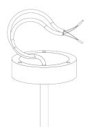
Gently remove the item from the package and proceed by screwing (clockwise) the black plate onto the tube (from the smooth side of the plate) into the relative thread.
