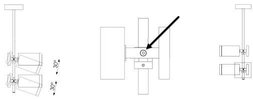
After that, adjust the side angle (left and right) of each satellite by regulating the screw located on the tube ring with a 4mm Allen wrench
