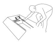
Firmly hold the metal pole and gently pull the lcarus\_Multiceiling out of the box.
