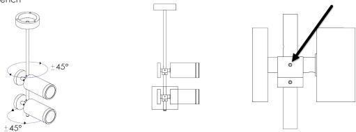
Make sure that both satellites and the two magnetic covers are securely and stably fastened.
